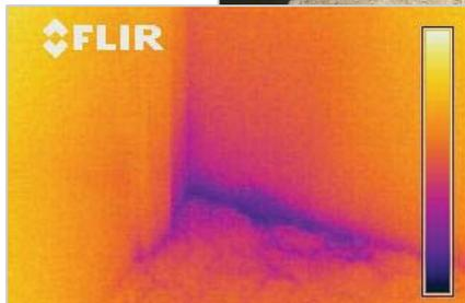
*By using infrared thermography we are able to pinpoint the location of water penetration into the wall and show area of saturation.* Further investigation revealed hidden fungal amplification both inside of the wall and under the carpeting. The problems were corrected and the odors were alleviated.
